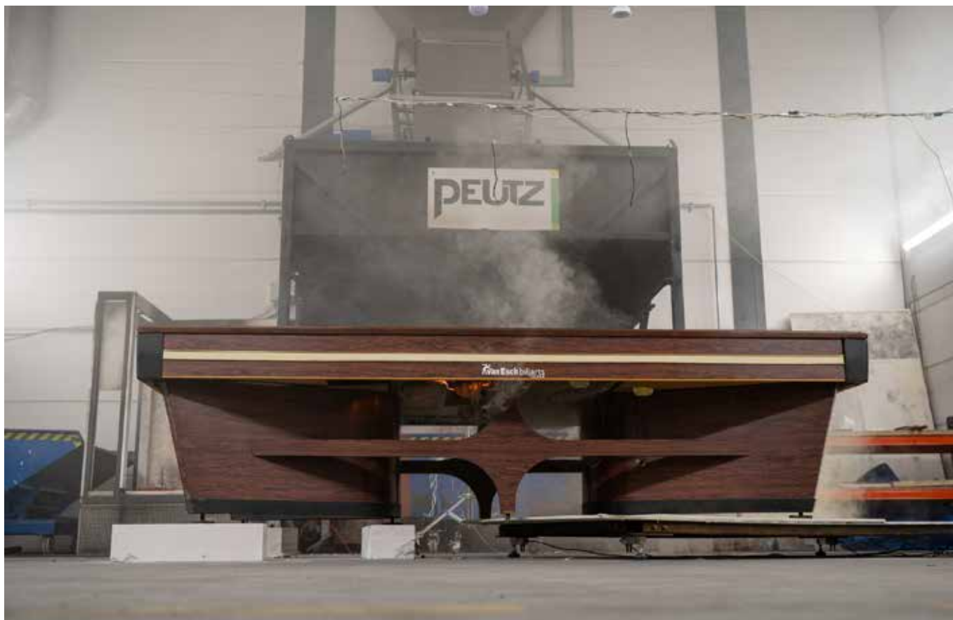
Figure 1. Full-scale fire testing of a billiard table at the Peutz laboratory.
