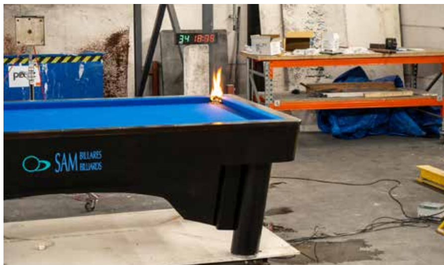
Figure 2. Full-scale fire testing of a billiard table at the Peutz laboratory.
