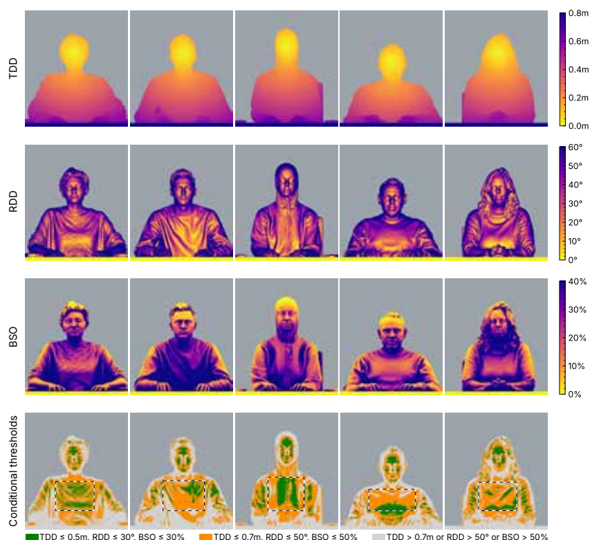
Figure 3. Dispersion of translational dosimeter displacement (TDD), rotational dosimeter displacement (RDD), and body self occlusion (BSO) factors impacting dosimeter performance on seated, screen-facing subjects.
