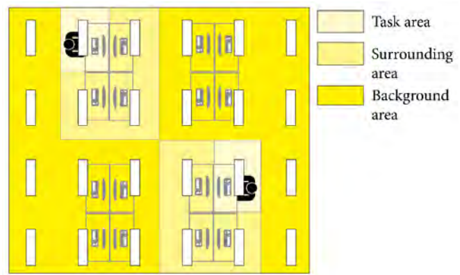
Figure 2. Concept of local lighting control for an example office case: different dimming levels in the task, surrounding, and background area when individual absences occur.
