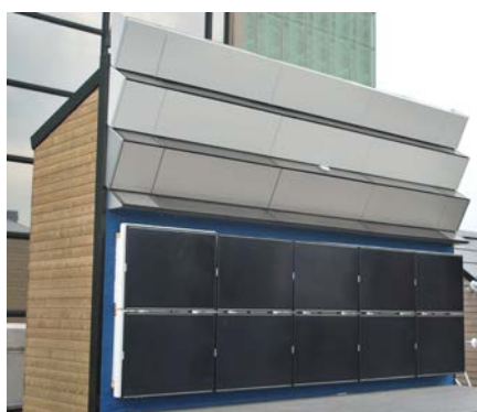
Figure 2. Picture of the façade cabin at which two companies of the ZonneGevel project are testing their new products. Lower part: SoloWall from SCX Solar. Upper part: ZigZag Solar from WallVision
