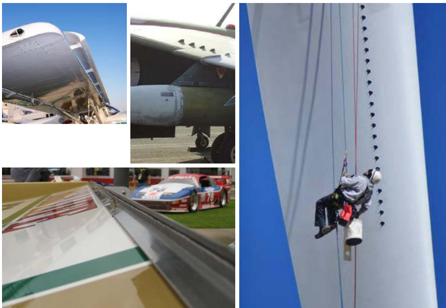
Figure 4. Leading-edge slot (top left) and vortex generator (top middle) on the aircraft wing; Gurney flap on Porsche 962 rear wing (bottom left); vortex generators on HAWT (right) [10]
