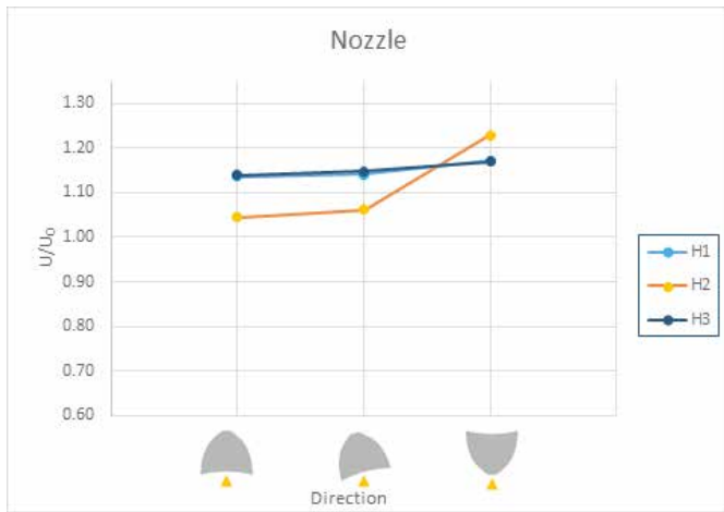
Figure 9. Wind amplification factors for nozzle configuration of duct for three wind directions (0, 15, and 180 degrees), H1–H3 – see Fig.6
