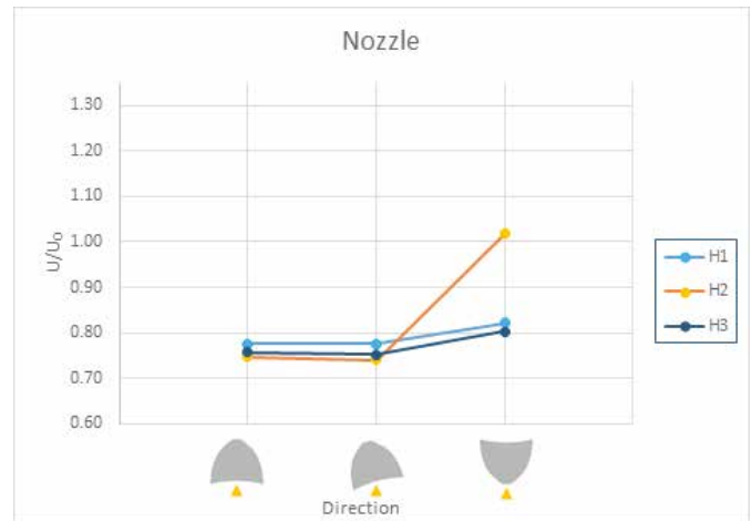
Figure 10. Wind amplification factors for nozzle configuration of duct for three wind directions (0, 15, and 180 degrees), H1–H3 – see Fig.6
