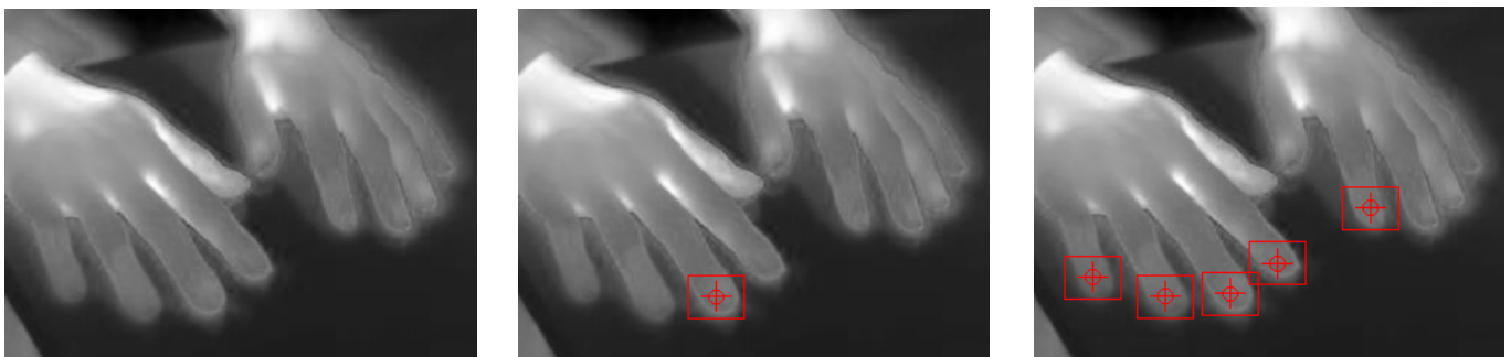
Figure 1 Pattern matching in a static image (from left: source image, marked pattern, matched patterns)
