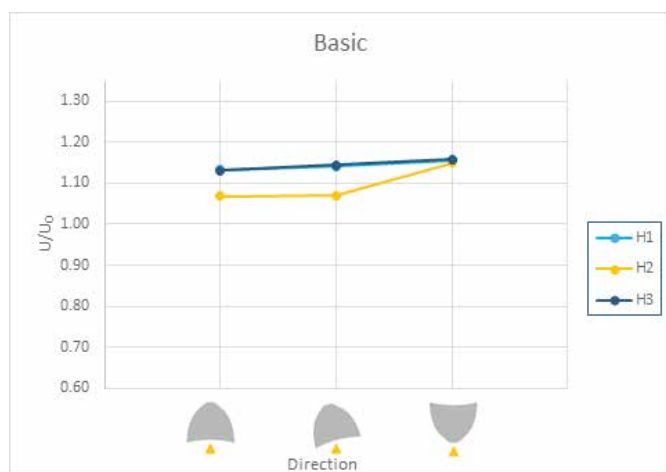
Figure 7. Wind amplification factors for basic configuration of duct for three wind directions (0, 15, and 180 degrees), H1-H3 – see Fig.6
