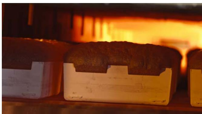
Figure 6 Moulds filled with FOAMGLAS® passing through the oven.
