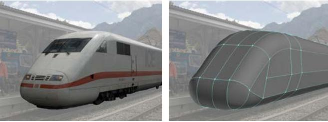
Figure 3 Mesh composition of the German ICE-2 train
