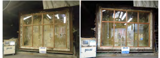
Figure 3 Experimental set up, double glazing (left) and triple glazing (right)
