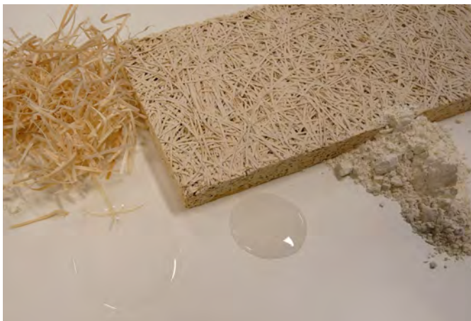
Figure 1 (L) A wood-wool cement board with ingredients like spruce wood-wool, cement, water and waterglass. (R) Wood-wool cement boards applied on ceiling for sound absorption.
